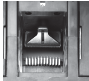
Magnum DS Breaker Contacts (Arc Chutes Removed)
