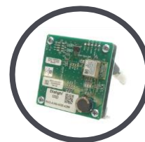
FLWIRELESS • Wireless controls card
